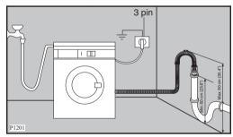
The drain hose may be extended to a maximum of 4 metres. An additional drain hose and joining piece is available from your local Service Force Centre. The joining piece must have an internal diameter of 18mm. If your drain hose looks like this (see below) you do not require the "U" piece". Just push the hose firmly into the standpipe.
